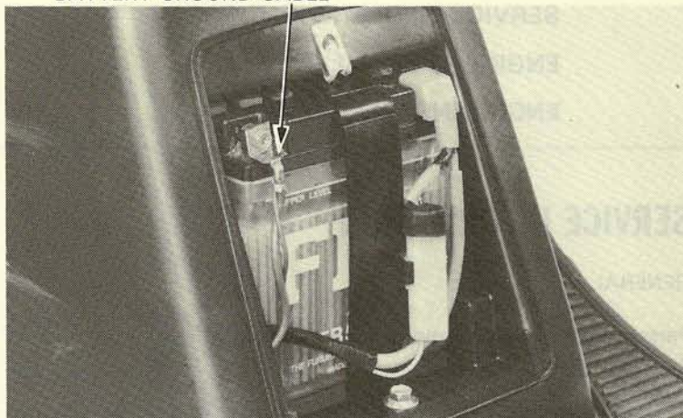
BATTERY GROUND CABLE
