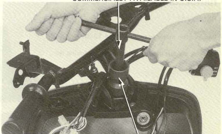
LOCK NUT WRENCH, 30 x 32 mm 07716-0020400 OR COMMERCIALY AVAILABLE IN U.S.A.
