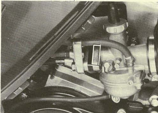
The carburetor identification number is on the left side of the carburetor body.
